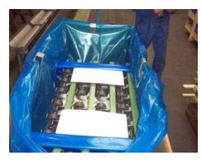
BRANOrost Chips are placed or hung in packaging or cavities with tightly sealed outer walls. The better the outer seal, the longer-lasting the protection. Depending on the size of the packaging, small-format chips such as cut-outs or punch outs can be used. Large-format chips are also available.
