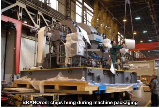
Protection duration : 3 years maximum in tightly sealed packaging. Depending upon climatic conditions BRANOrost R-Chip : Recommended for Steel, cast iron, chrome, block tin, high-grade aluminium.
